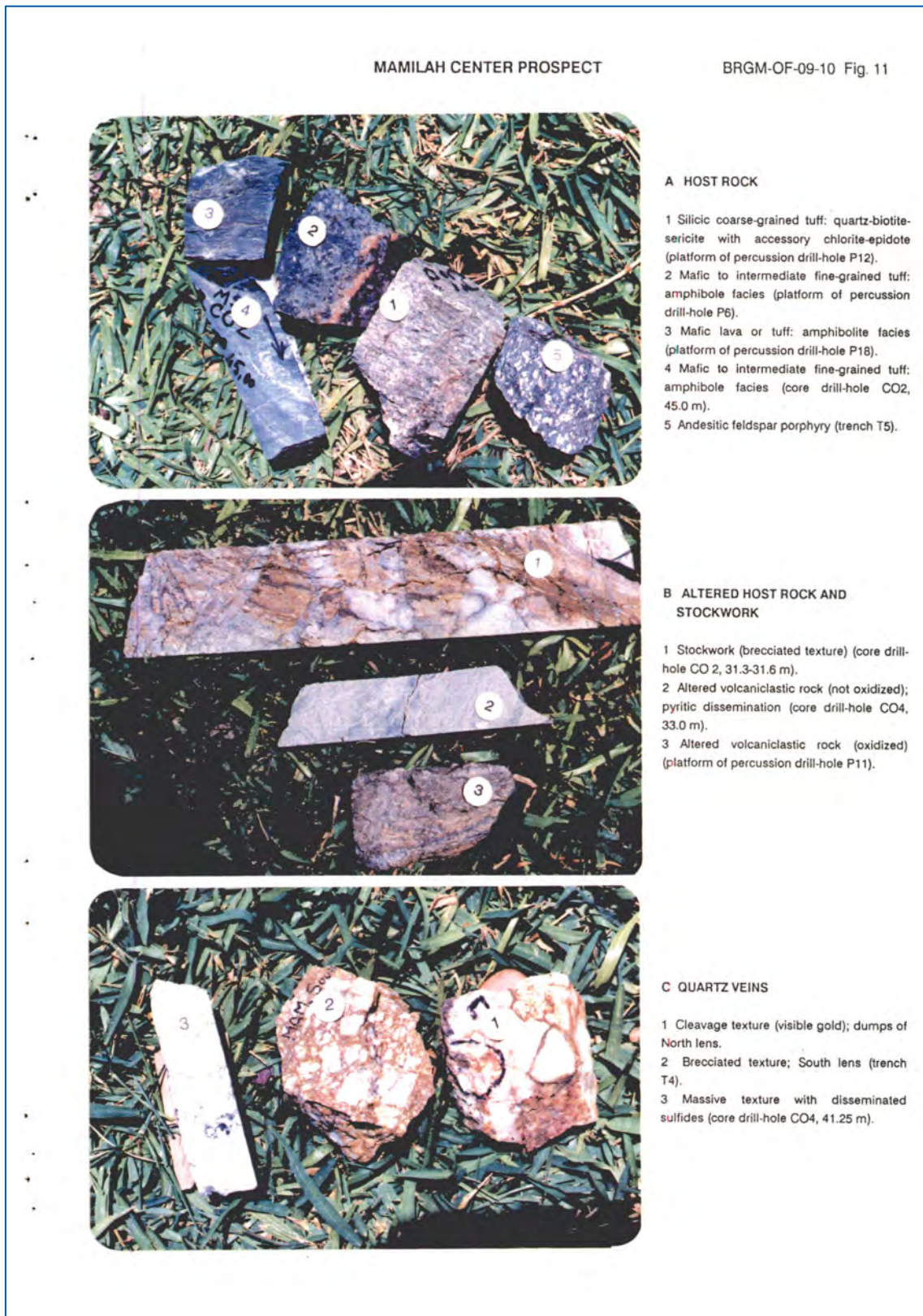
Figure 8: Core and Grab Samples photos from Mamilah Center Prospect
