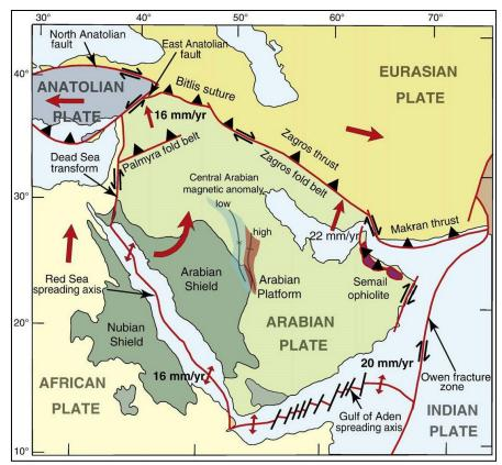
Figure 2: Tectonic framework of the Arabian Peninsula, showing plate boundaries, relative plate motion vectors, and major fault zones (Stern and Johnson 2010).
