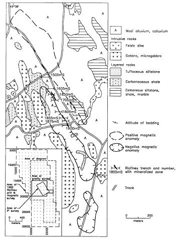
Figure 8: Geology of Al Miyah prospect showing Riofinex trenches and magnetic and gravity anomalies. Modified after Sheppy (1983).
