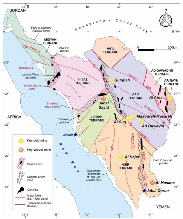
Figure 4: Simplified geological map of the Arabian Shield, showing the locations of key mines within the Kingdom. Major tectonostratigraphic terranes are delineated by sutures and major fault zones. Al Miyah is located within the Asir Terrane, toward the southeastern corner of the map. Modified after Nehlig et al. (2002).
